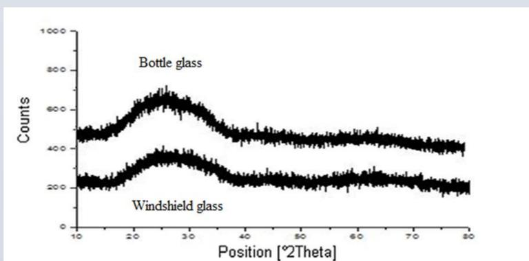
Fig. 1. X-ray spectrum of waste glasses.
