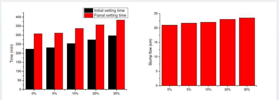
Fig. 2. Setting time of cement mortar samples. Fig. 3. Slump flow of cement mortar samples.
