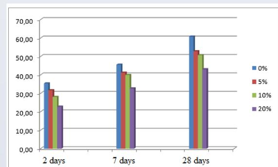
Fig. 3. Compressive strength of cement mortars samples
