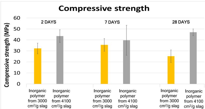
Figure 3 - Compressive strength Analysis
